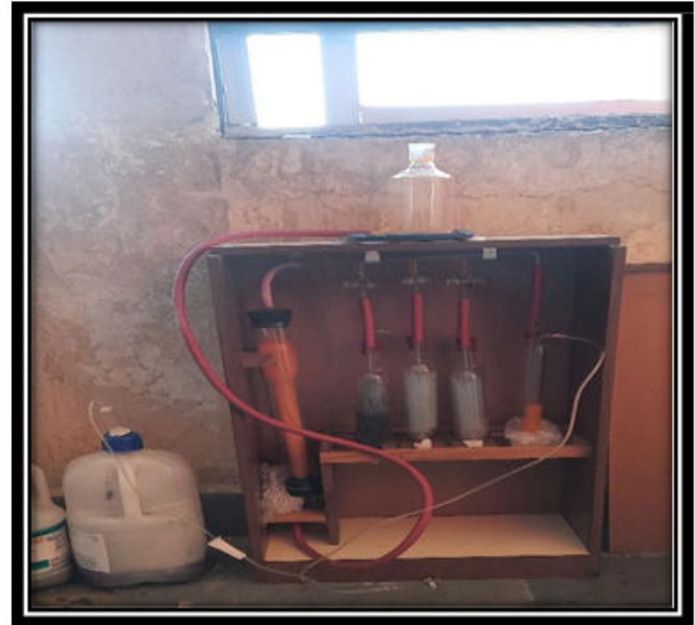
Figure 3. Orset method for biogas measurement.
