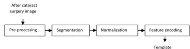
Figure 2. Illustration of iris template generation.
