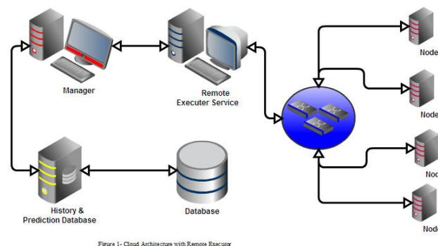
Figure 1- Cloud Architecture with Remote Executor
