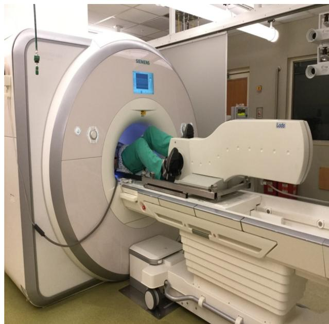
**Figure 1.** Positioning for cycle exercise within the MRI scanner. The chest remains within the magnet bore for image acquisition while the feet are secured to the pedals of the MRI-compatible cycle ergometer.
