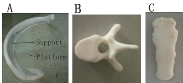
**Figure 1.** a); The rib after 3D printing b); Thoracic vertebra c) Sternum.
