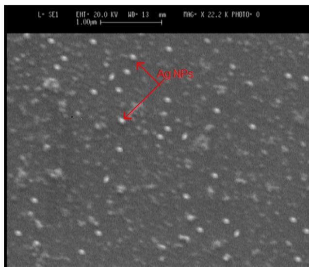
**Figure 1.** Electron microscope image of biosynthesized silver nanoparticles.
