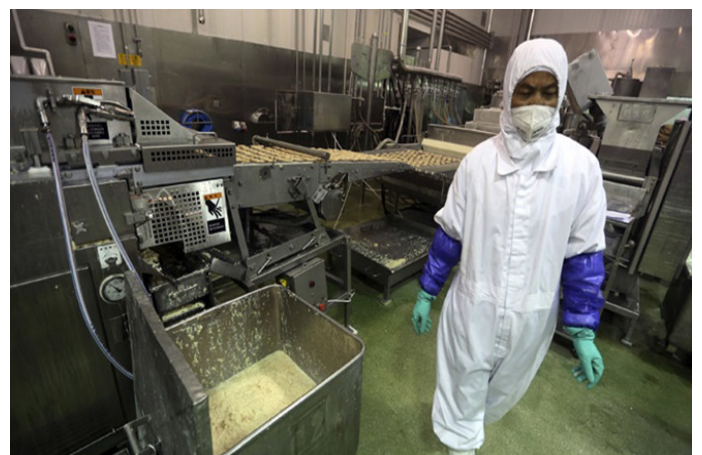
Figure 4. Butter filtration unit.
