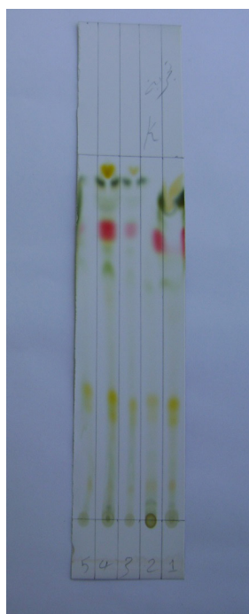
Figure 3. Thin layer chromatography plate during the process of separating some oxygen terpenes of the genus Potamogeton using the solvent (Ethyl acetate-chloroform, 10-90,v/v) as a mobile phase.
