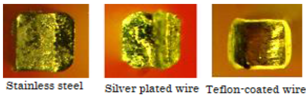
Figure 1. Sectional view of sample wires. The samples are from left Stainless steel, Silver plated wire, and Teflon-coated wire.
