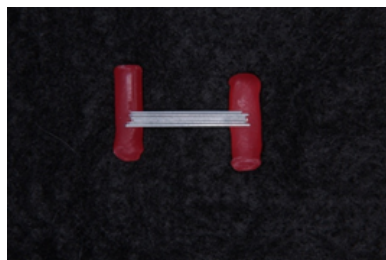
Figure 5. Sample wire segments in color measurements. Wire segments were placed tightly at both ends and fixed with wax.
