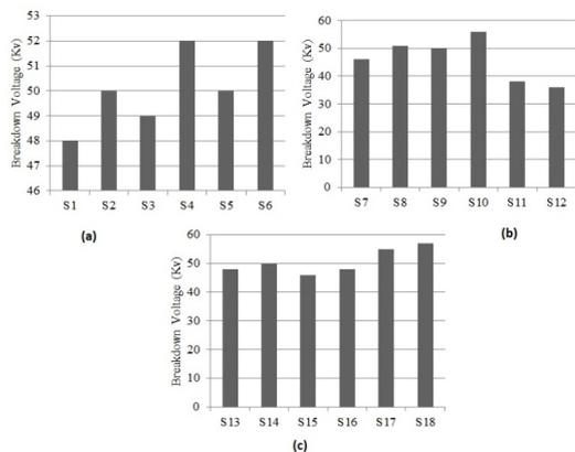
**Figure 2.** (a). Breakdown voltage characteristics of base fluid-1 with Butylated Hydroxyanisole (BHA), Butylated Hydroxytoluene (BHT) and Propyl Gallate (PG) antioxidants. (b). Breakdown voltage characteristics of base fluid-2 with Hydroxyanisole (BHA), Butylated Hydroxytoluene (BHT) and Propyl Gallate (PG) antioxidants. (c). Breakdown voltage characteristics of base fluid-3 with Hydroxyanisole (BHA), Butylated Hydroxytoluene (BHT) and Propyl Gallate (PG) antioxidants.
