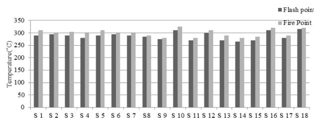
**Figure 4.** Flash and fire point characteristics of base fluids 1, 2 and 3 with antioxidants.
