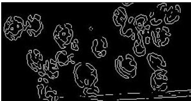
Figure 9. LoG operator-output image.
