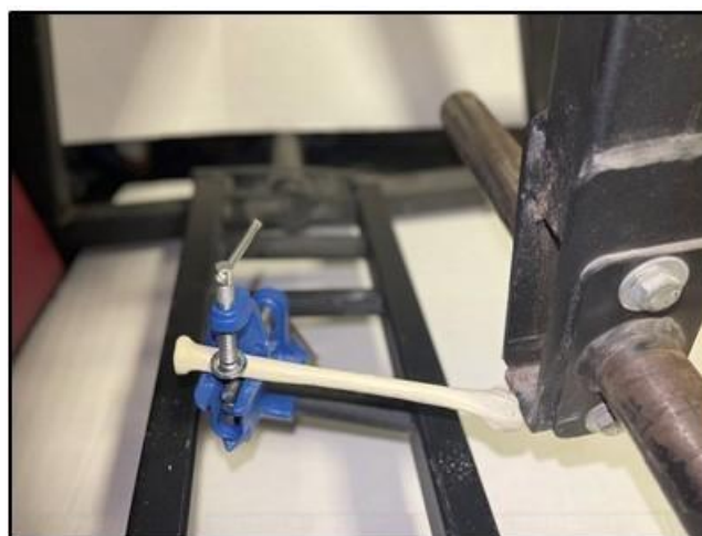
Figure 2. Radius was placed into a clamp holding the proximal radius and at 80 degrees of inclination to the point of impact of the force vector. A swingarm with a weight on the end was employed to simulate the rotational fall onto an outstretched hand.
