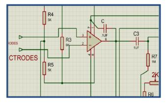
Figure 2. First stage of amplification.
