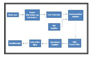
*Figure 1.* Block diagram of the EEG circuit. The circuit consists of three parts: acquisition, amplification and filtering.
