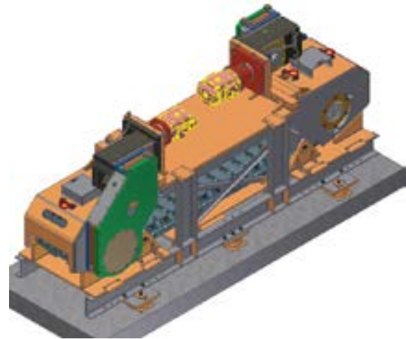
Figure 2: Describe the traction reducer test bench fully assembled
