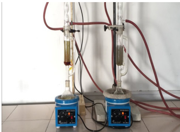
Figure 4. Soxhlet apparatus using phytochemical extraction.
