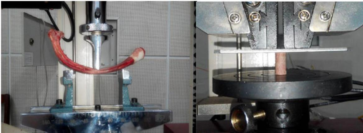
**Figure 7.** The left panel was the picture of the three-point bending test for the measurement of material parameters of the rib; the right panel was the picture of the compression test for the measurement of material parameters of the vertebrae.
