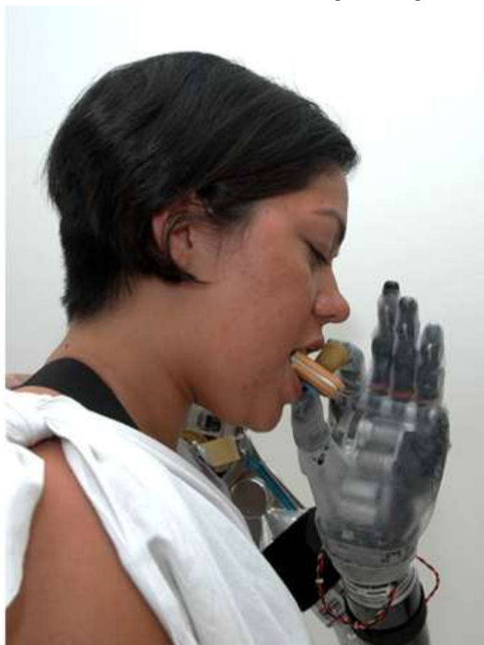
Figure 3. Two targeted reinnervation patients perform functional manipulation tasks with an advanced prosthetic arm. Photos courtesy of the Rehabilitation Institute of Chicago and DEKA Research.
