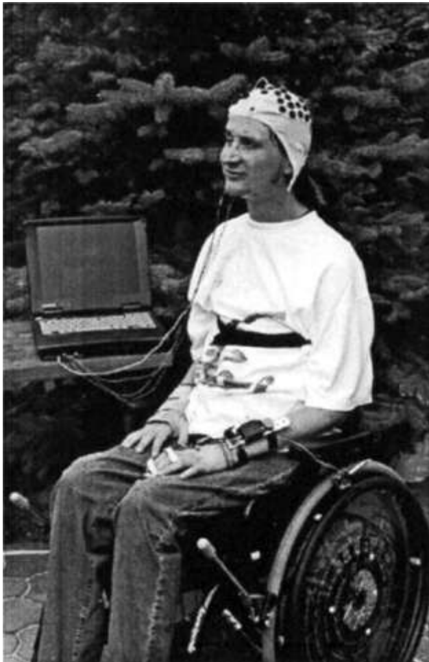
Figure 9. An EEG system recording mid-frequency signals is used to control a hand orthosis. Reprinted from Pfurtscheller et al [92], Copyright © 2002, with permission from Elsevier.
