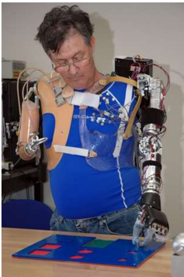
Figure 3. Two targeted reinnervation patients perform functional manipulation tasks with an advanced prosthetic arm. Photos courtesy of the Rehabilitation Institute of Chicago and DEKA Research.
