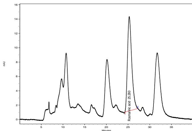
Fig 5: HPLC chromatogram of rosmarinic acid in EEOS.
