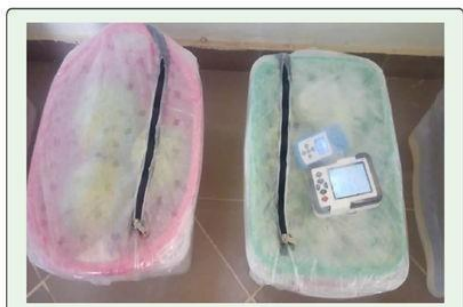
Figure 1. The setup of HMAS with oxygen and carbon dioxide readers.
