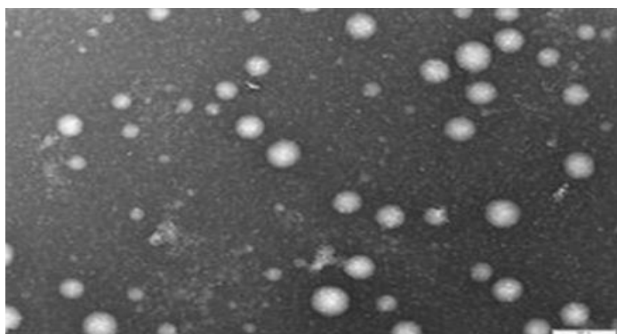
Figure 1. Image by transmission electron microscopy TEM of a granule internal section where nanoliposomes are visible, with
