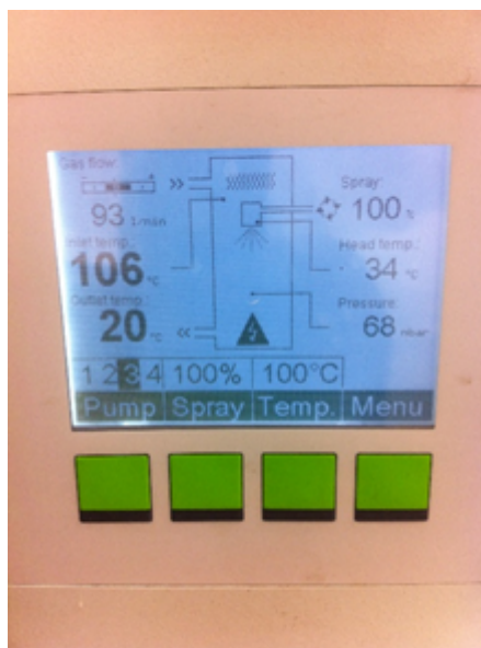
Figure 4. Buchi B-90 nano spray drying showing process parameter settings.
