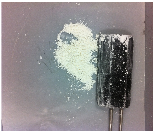
Figure 2. Spray dried nano particles showing rubber spatula and loss during collection.
