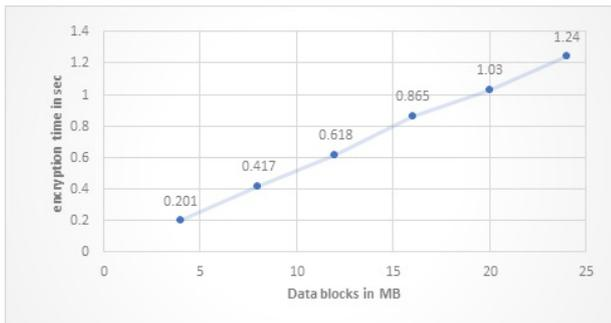
Figure 3b. Performance of Encryption time.
