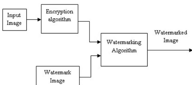
Figure 1. Basic model for Copyright protection.
