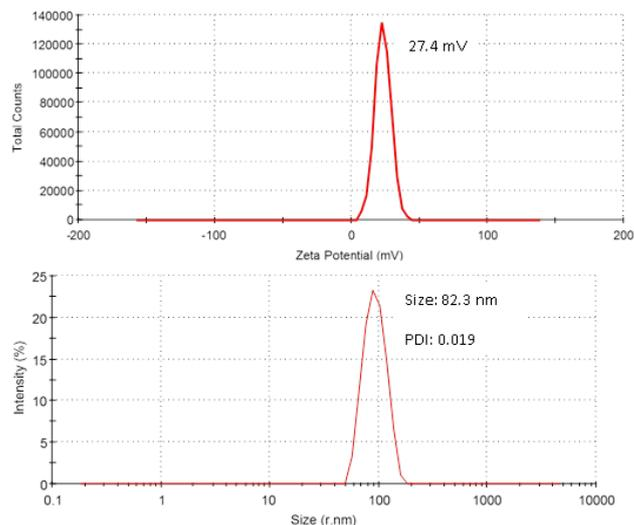
Figure 2. Characteristics of the developed DCNPS i.e. zeta potential and particle size.
