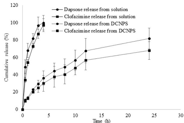
**Figure 3.** In vitro dapson and clofazimine release study from DCS and DCNPS in PBS 7.4 pH.
