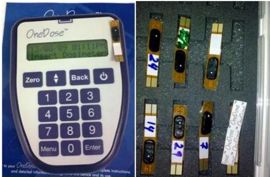
**Figure 2.** (Left) the OneDose system with the detector, (Right) close-up of the detector.
