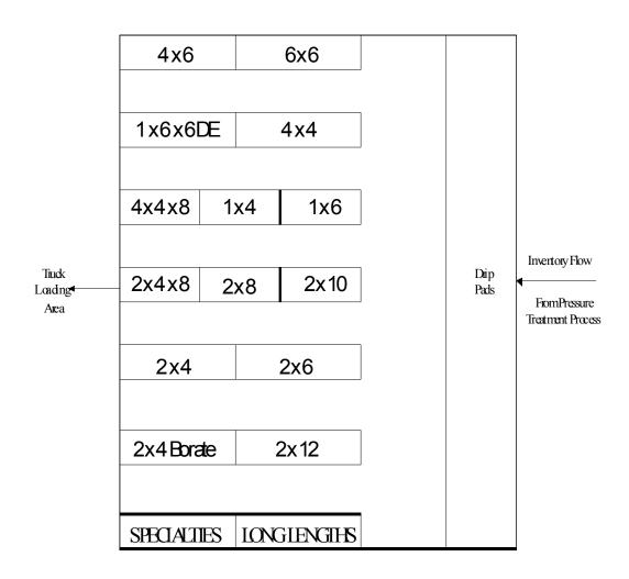
FIGURE 4 – Modified Warehouse Layout
