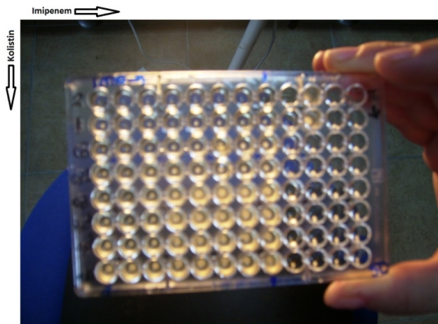
Figure 1: Colistin-imipenem combination and checkerboard method.
