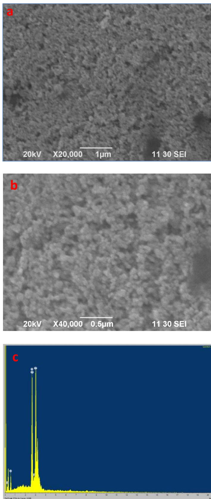
**Figure 4.** SEM micrograph showing the morphological characteristics of silver nanoparticles synthesized using leaves of *C.gigantea* leaf extract. **a.** Lower magnification. **b.** Higher magnification. **c.** EDX showing the chemical constituents of the synthesized nanoparticles.
