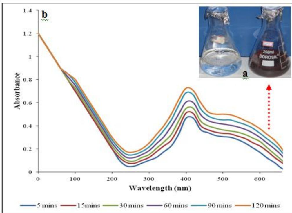
**Figure 2.** a Aqueous solution of AgNO<sub>3</sub> with *C.gigantea* leaf extracts (left) before adding the leaf extract and (right) after addition of leaf extract at 120 min. b UV-Vis spectra of aqueous silver nitrate with *C.gigantea* leaf extract at different time intervals.
