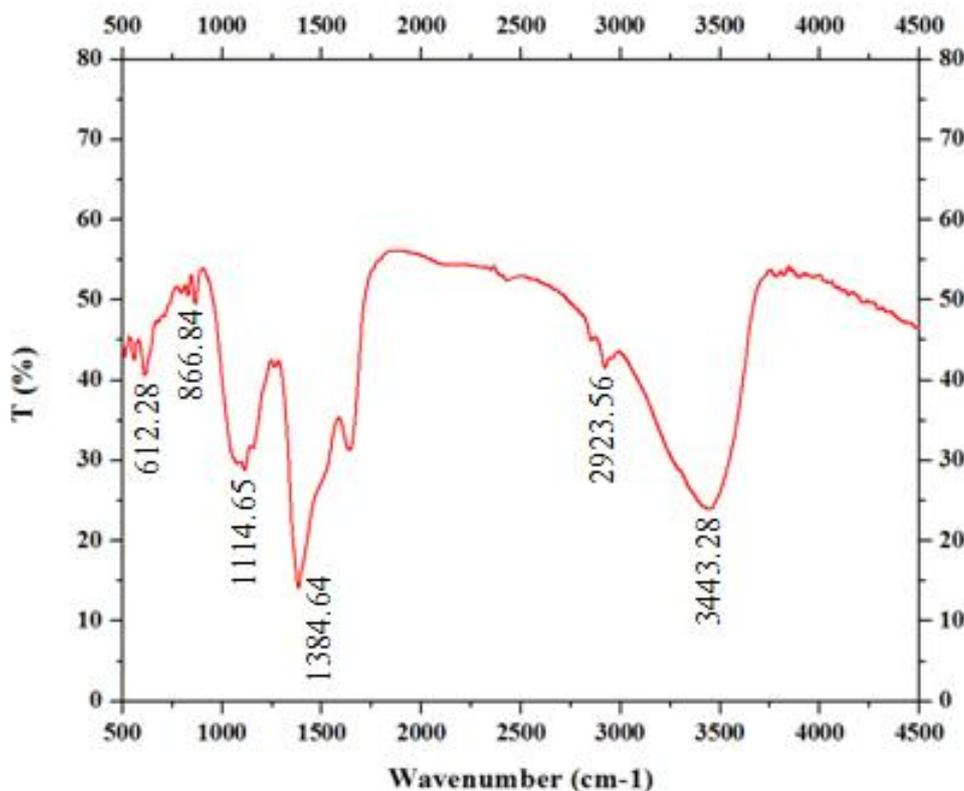
**Figure 3.** FTIR spectra of vacuum-dried powder of synthesized AgNPs from *C.gigantea* leaf extract.
