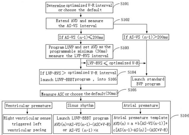
Figure 3. Algorithm of BVR realized by LUVB-BBTT.
