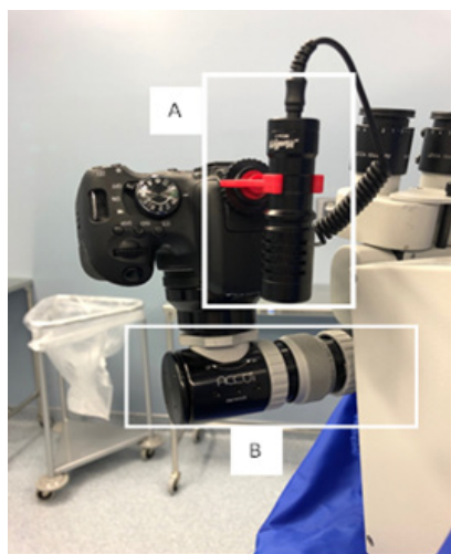
Figure 1. Camera and microphone attachments. 1A: Moukey MCM-1 microphone attached and plugged into the Canon T5I DSLR camera; 1B: Camera adapter (TTI Medical) to transmit surgeon's view.
