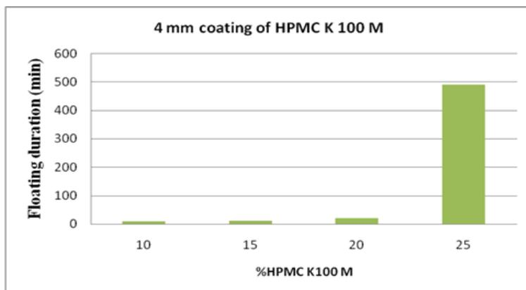
Figure No.6. Effect of polymer concentration and coating level on floating duration
