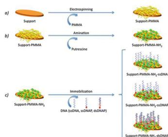
**Figure 3.** Electrospinning fabrication technique
