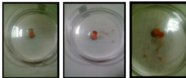
Figure No 3: Side view of bust release of dug from rupturable coating. After erosion of ethyl cellulose medium get contacted with inner swelling layer of croscarmellose sodium (Ac-Di-Sol) bust effect on coating layer give rapid drug release.
