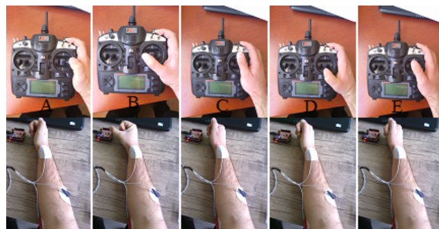
Figure 2. Thumb gestures both remote controller and EMG acquisition system. A) Right B) Left C) Forward D) Backward E) No movement.
