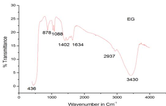
**Figure.6.** shows the FTIR spectra for the ethylene glycol medium.
