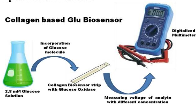
**Figure 4** shows the experimental methodology applied.
