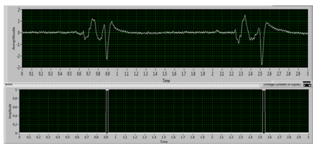
Figure 11. Shows the output from the amplifier of the two eye blink and its corresponding pulses for control.
