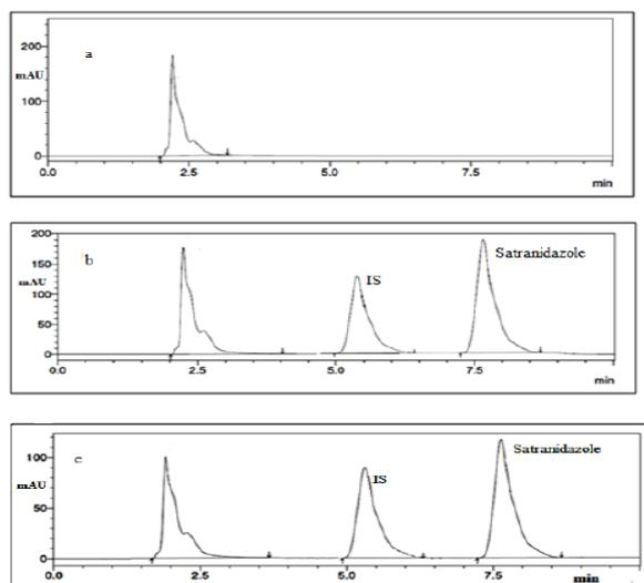
**Figure 2** HPLC Chromatograms of 20µL injection of a. blank plasma; b. blank plasma spiked with satranidazole (70µg/mL) and IS (35µg/mL); c. plasma sample at 3h after oral administration of satranidazole at a dose of 50 mg/kg to rats. The retention time of satranidazole and IS were 7.7 min and 5.5min respectively.
