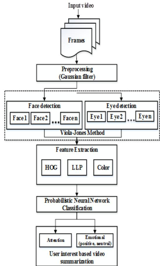
Figure 1. Flow diagram of MFE-VS.
