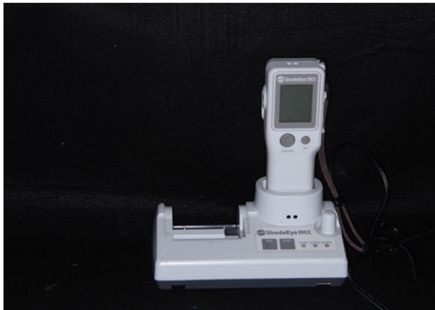
Figure 3. Colorimeter used in the study (Shade Eye, Shofu, Kyoto, Japan). In this colorimeter, the value of L was measured lightness ( L^* ) and Hue ( a^* \cdot b^* ).
