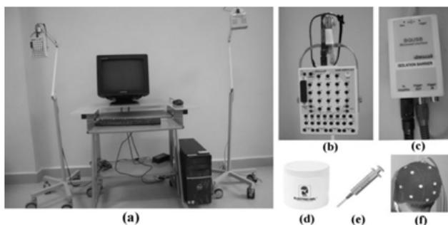
**Figure 1.** EEG data acquisition system, (a) full equipment, (b) Amplifier; (c) Isolation barrier; (d) Electrode gel, (e) Gel injection syringe, (f) Electrode hat
