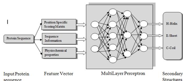
Figure 3. Proposed architecture of multilayer perceptron classifier.
