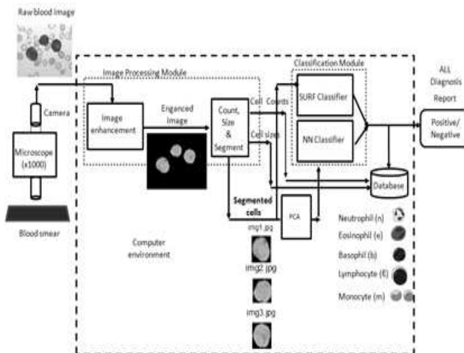
**Figure 1.** Block diagram representation of overall process
