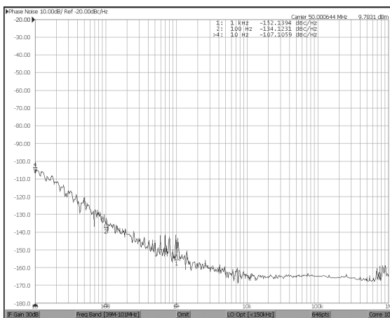
Figure 6. Measured phase noise curve after adjusting C_2 .
