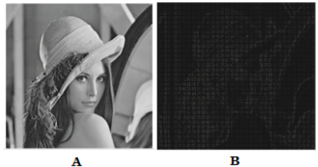
Figure 5. (a) Gray-scale image of lena; (b) Edges of the image lena detected by sobel technique.
