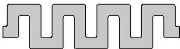
Figure 2. Meander shaped microfluidic Channel.
