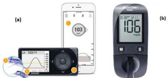
Figure 1: (a) Dexcom G5 CGM system, (b) Accu-Chek active blood glucose meter [1,2].
