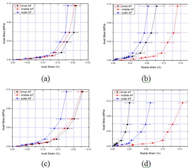
**Figure 3.** Stress-strain curve of the intervertebral disc under compression load. (a) Axial stress-axial strain curve in anterior AF; (b) Axial stress-radial strain curve in anterior AF; (c) Axial stress-axial strain curve in posterior AF; (d) Axial stress-radial strain curve in posterior AF.
