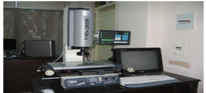
Fig 1. Computer vision system for acquiring images
