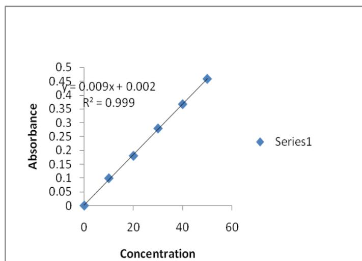
**Figure 2:** Calibrated Curve for Tizanidine Hydrochloride at 617 nm
