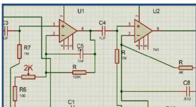
Figure 3. Second stage of amplification.
