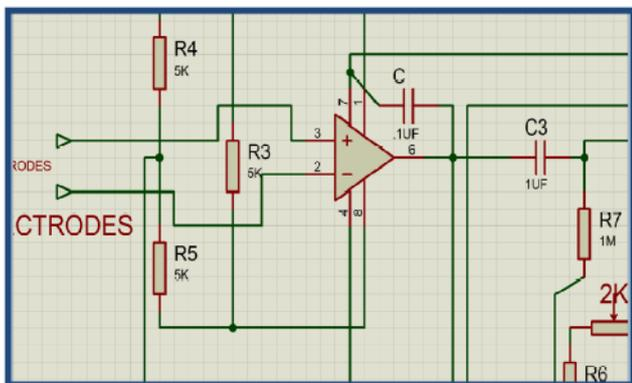
Figure 2. First stage of amplification.
