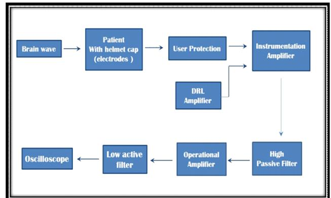
Figure 1. Block diagram of the EEG circuit. The circuit consists of three parts: acquisition, amplification and filtering.
