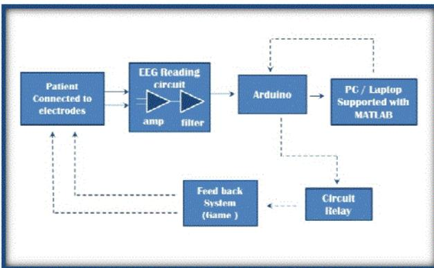
Figure 8. Block diagram of the project.
