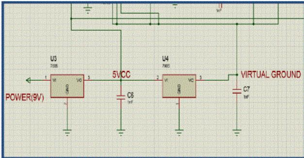
Figure 7. Power supply and VGND.
