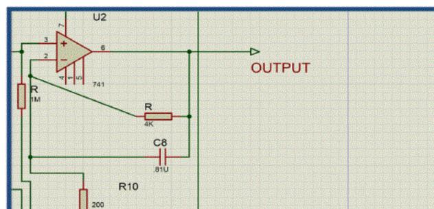
Figure 4. Third stage of Amplification.
