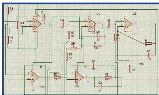
Figure 5. All stages of amplification.
