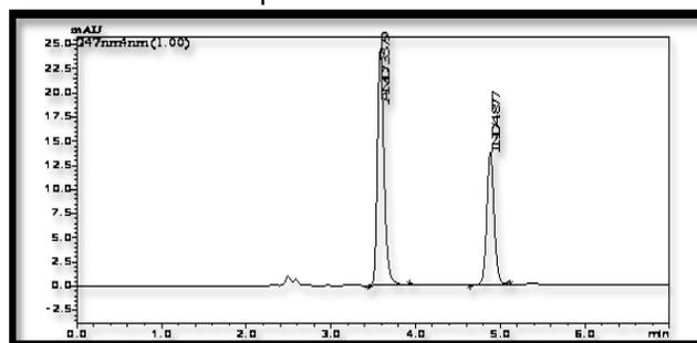
Figure 4.A typical chromatogram of standard solutions of AMD and IND
