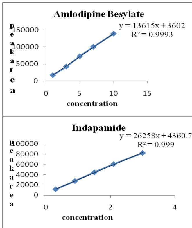
Figure 5.Calibration curve of AMD and IND
